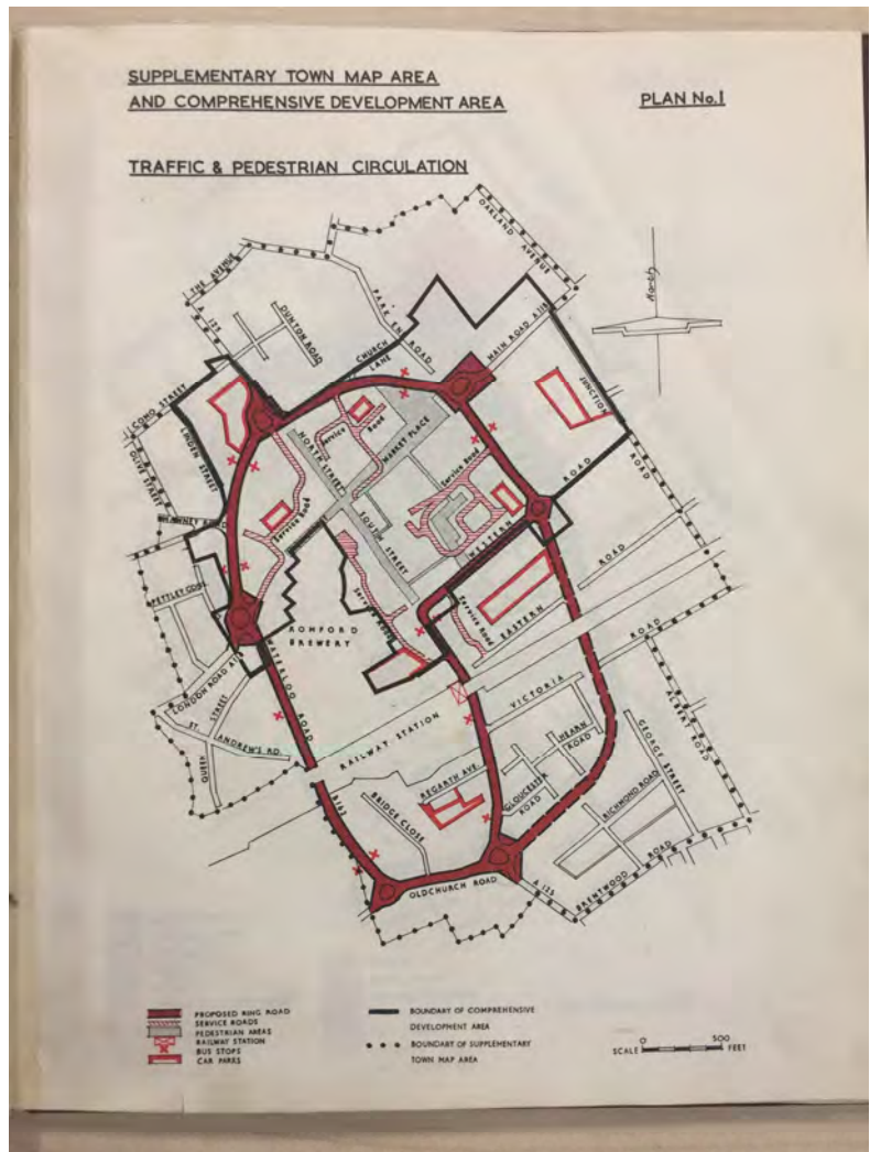
The movement plan envisaged with ring road around the town centre north and south of the railway and segregated central zone.
